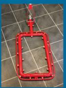
Fire hose C-2" is connected and at 4 bar water pessure each unit produces water mist with min. 137 Litres per minute for effective cooling of the batteries, as well as extInguishing open flames.
