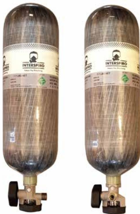
All Interspiro cylinder valves include a pressure gauge, an upstream connected safety relief valve disc. The diamond shaped hand wheel gives easier handling when wearing gloves and prevents accidental closure of the valve.
