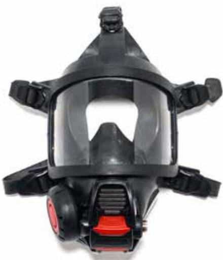
As soon as the breathing valve is connected to the Inspire-A Automatic mask it is activated and the mask is ready for use without any additional measures. The quick connection makes installing and removing the breathing valve very easy. To install the breathing valve, it is simply pushed into the mask and locks in place. To remove it, the two red buttons are pressed simultaneously and the breathing valve pulled out from the mask.
