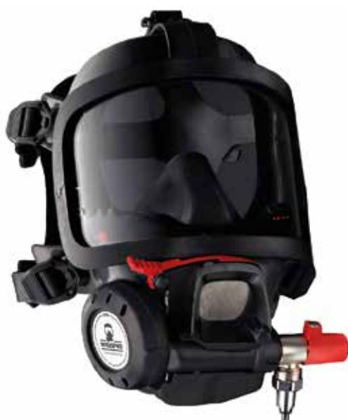
The mask is equipped with an ambient air hatch enabling the user to have the mask fully donned and still breathe ambient air to save the compressed air in the cylinder. With a very simple operation, a push on the hatch cover, the air from the cylinder is activated.
